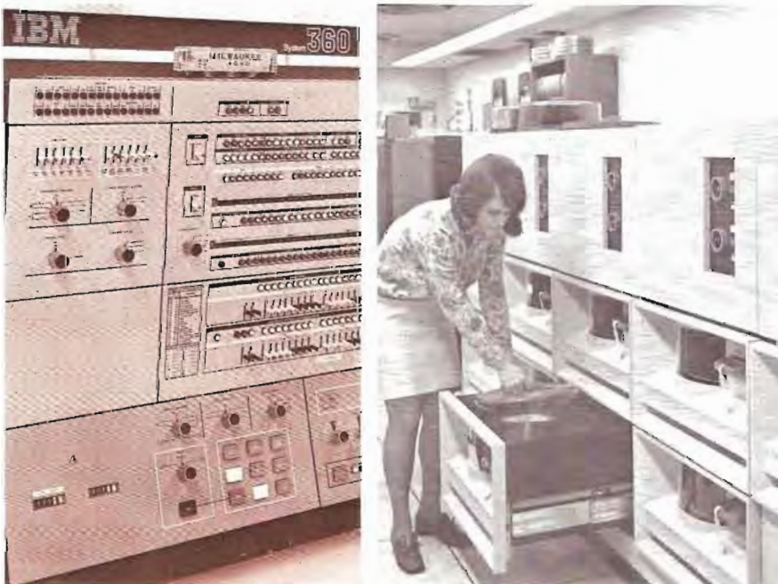
The IBM 360, model 40 (lower left) was installed to update Carscope, the railroad's car reporting center. Magnetic disk data storage units are shown at lower right.
