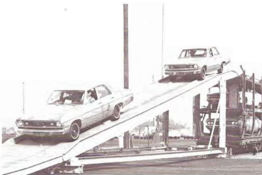
New automobiles being unloaded from tri-level automobile rack cars in the automobile marshaling complex at Kent, Wash.
