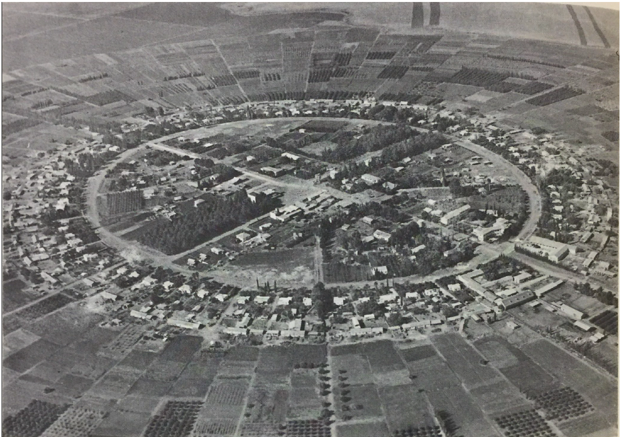
Figure 4 The layout of Nahalal, a moshav in the Galilee region, reflects its defensive purposes, with public buildings and stores in the middle, farmhouses around that, and agricultural fields forming a perimeter. (Weintraub et al., 1969).
