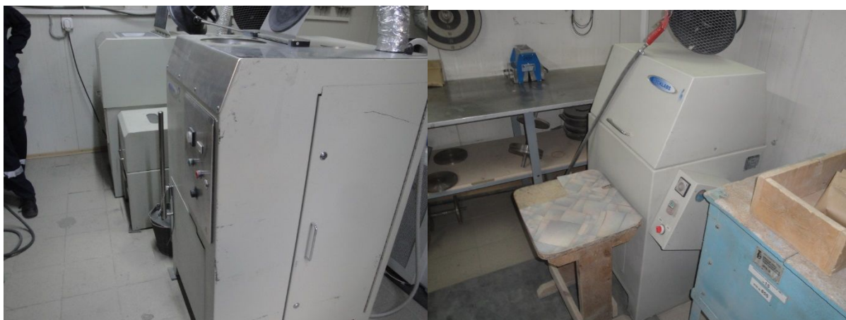
Photo 10.3: Rocklabs Mill Equipment used for Sample Preparation
