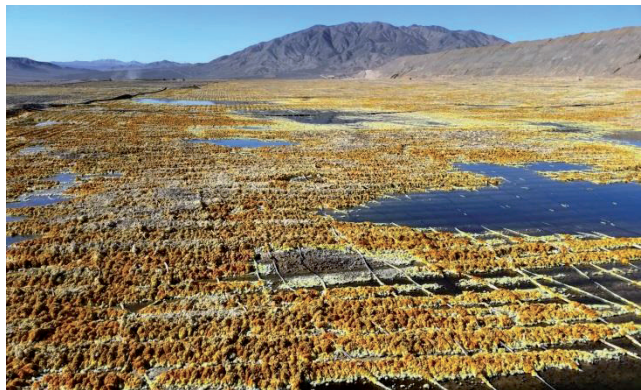
Figure 6. Leaching heap with water puddles and efflorescents.
