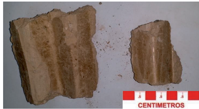
Figure 5. Material jammed in the crushing line.
