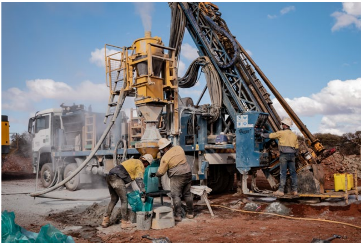
Reverse Circulation drilling for the Moolart Well expansion
