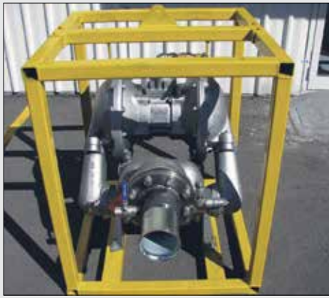
Custom-built sets of new Sandpiper pumps, housed in frames, offer a creative solution for a tough, portable rig, painted to customers specifications.
