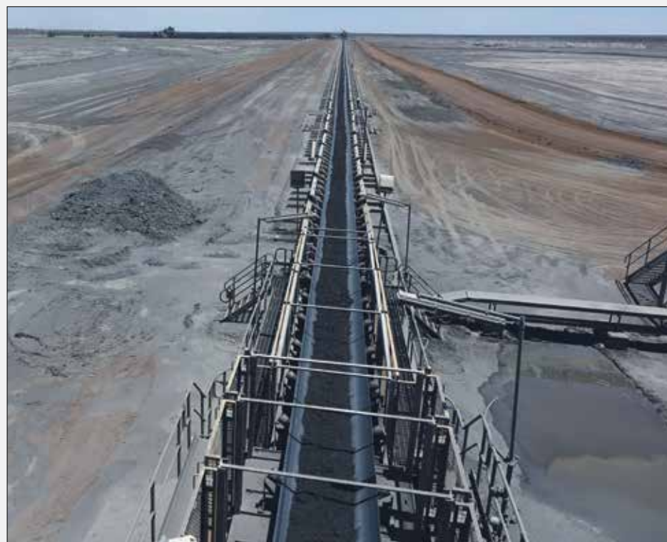
The modular conveyor can be elongated or reduced to suit production.
