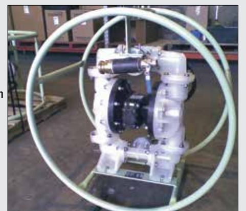
The set-up of the Sandpiper 1", 2", and 3" air-operated diaphragm pumps in roll frames is more versatile than other builds and could suit a better range of potential applications.
