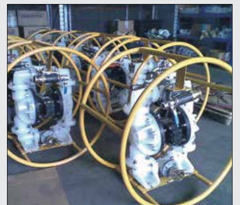
The Sandpiper HD20F plastic bodied (non-metallic) flap-check valve pump is an ideal pump for harsh mine dewatering applications: one that is lightweight, resistant to corrosion, easy to maintain as well as able to pass large solids through the system.
