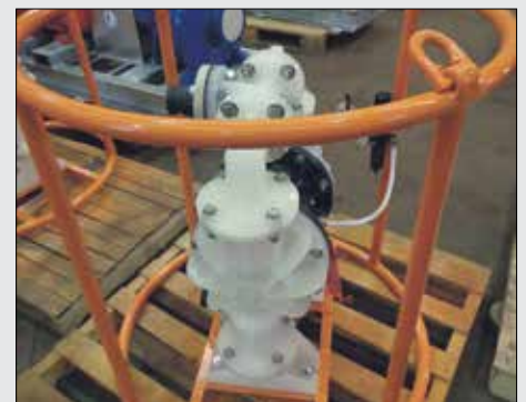
Lifting lugs can be included on cages/frames to lift them on and off the trucks and onto sites easily and safely.
