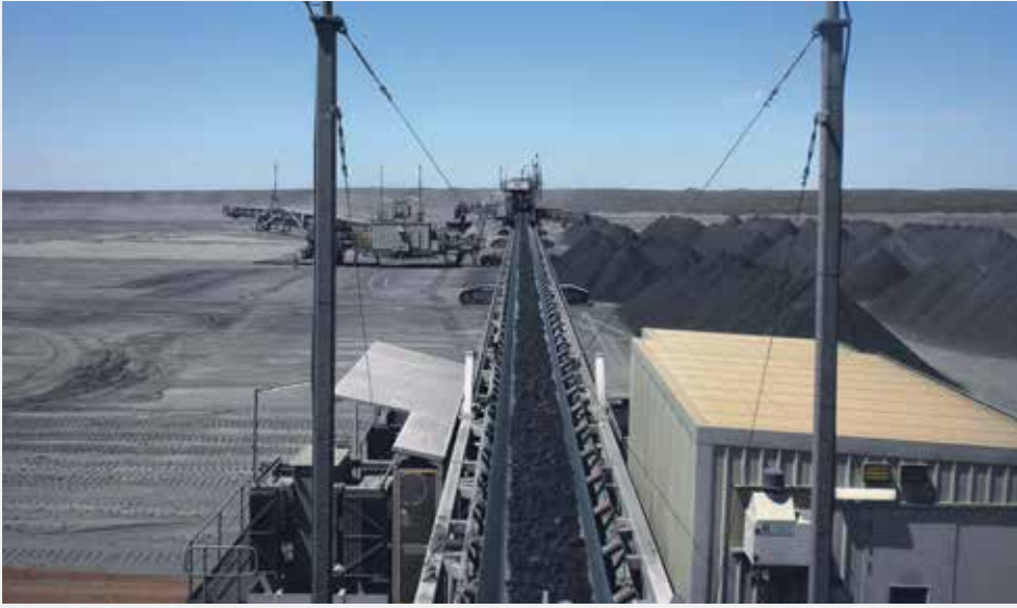
Stacks fit into a 2km x 2km footprint, layered up to 90m high.
