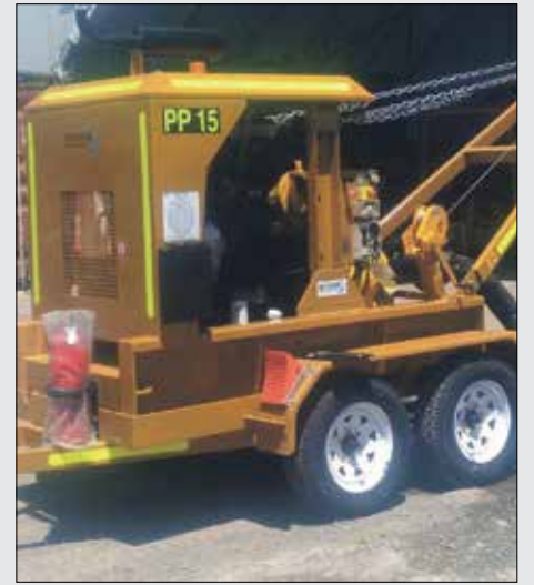
The components were blast and painted, pump wet-end overhauled and the engine tested and serviced.
