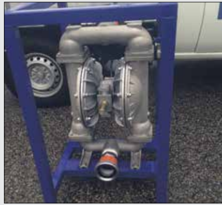
Custom-built sets of new Sandpiper pumps, housed in frames, offer a creative solution for a tough, portable rig, painted to customers specifications.
