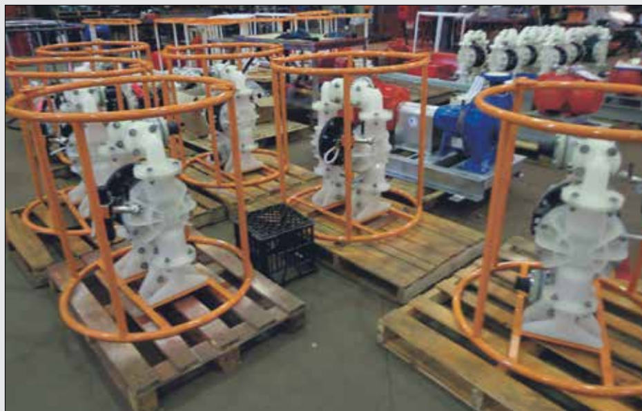
The set-up of the Sandpiper 1", 2", and 3" air-operated diaphragm pumps in roll frames is more versatile than other builds and could suit a better range of potential applications.
