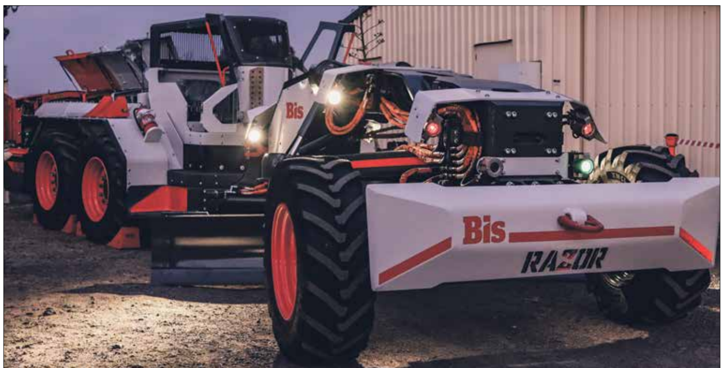
The key features of Razor include superior engine power and grader mass that has been optimised to increase tractive effort by more than 30pc.
