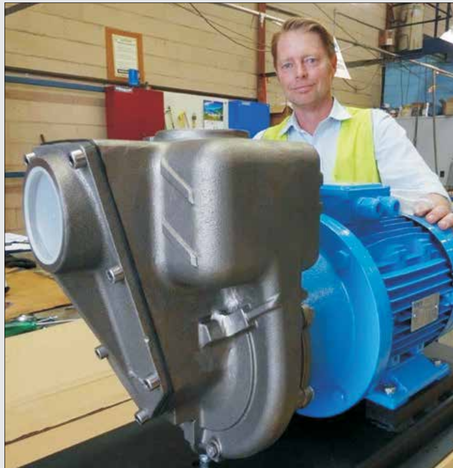
The Corrosive liquid mine pump G3TMK-A/ST, when applied to a tanker, is vital for dust suppression on mining sites during dry and windy seasons.
