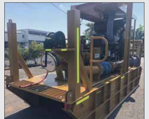
The pump skid after the Scope rebuild.
