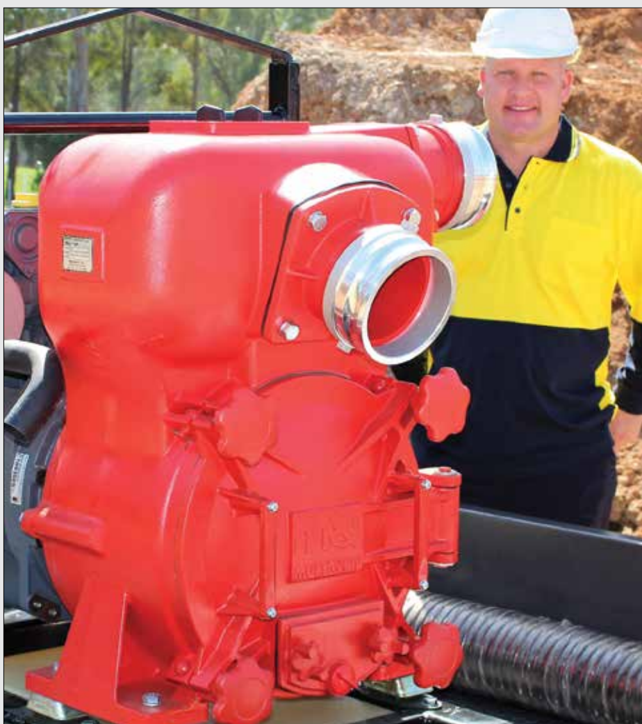
Ideal for site dewatering in mines and quarries, Aussie's new Kubota powered six inch trash pump can be mounted on a trailer or transported by utility vehicle.
