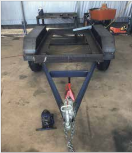
A heavy duty mining spec trailer was built for the pump.
