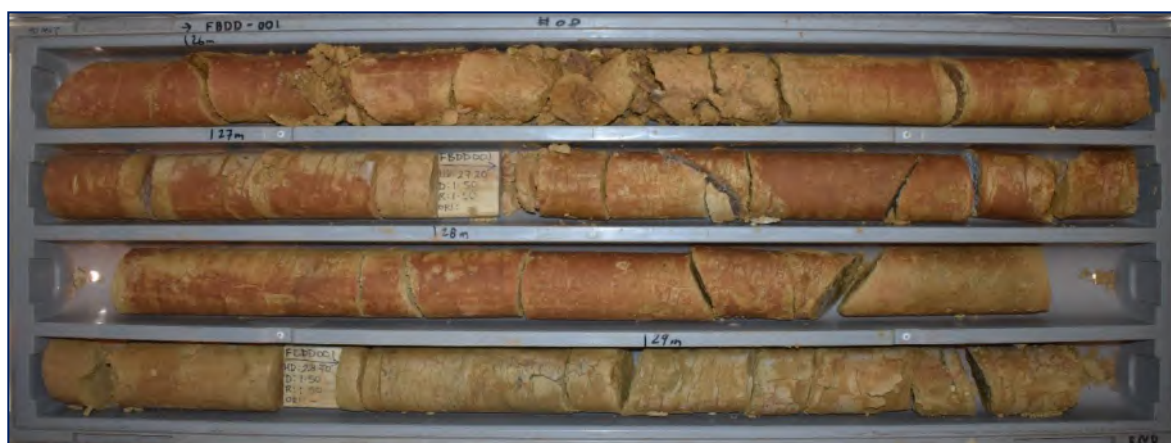
Plate 2 FBDD001 25.9m – 29.5m extremely/ highly weathered UZZ very poor quality material
