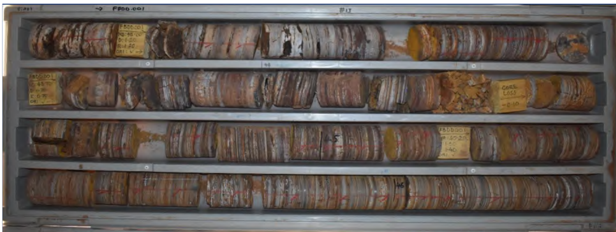
Plate 3 FBDD001 42.9m to 46.3m slightly weathered SIF fair quality rock
