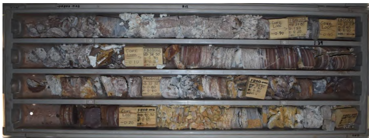
Plate 4 FBDD002 37.0m to 40.8m altered/ sheared breccia chert/ SIF poor quality rock
