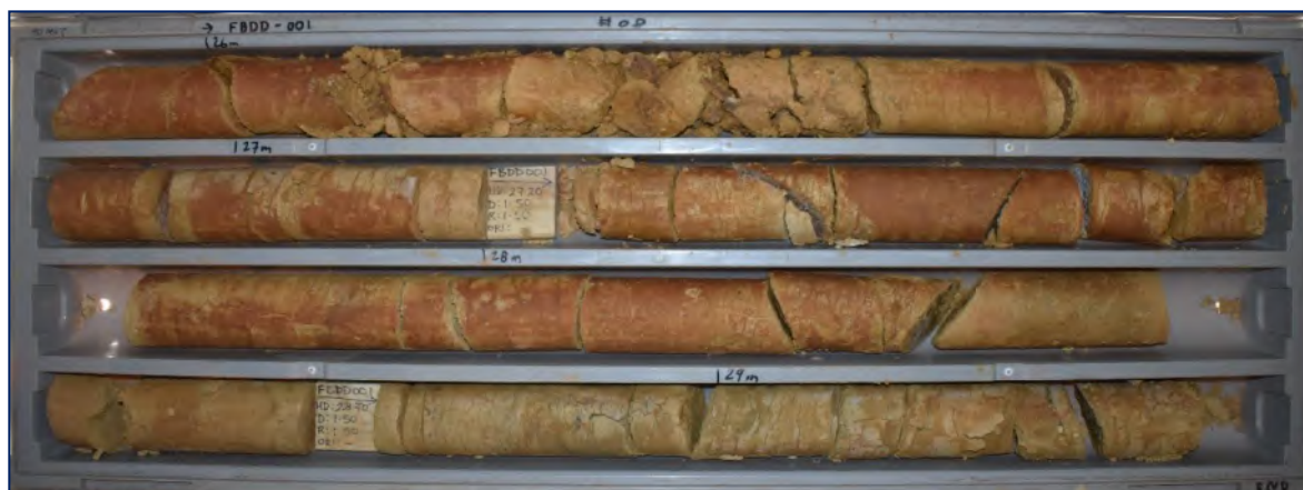
Plate 2 FBDD001 25.9m – 29.5m extremely/ highly weathered UZZ very poor quality material
