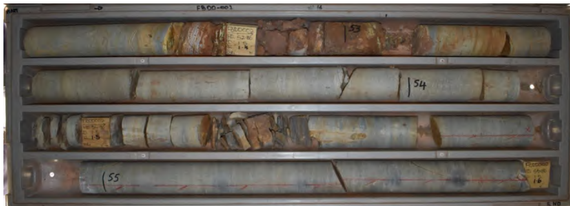
Plate 5 FBDD002 52.3m to 55.8m moderately weathered to fresh SIF and dolerite poor to fair quality rock
