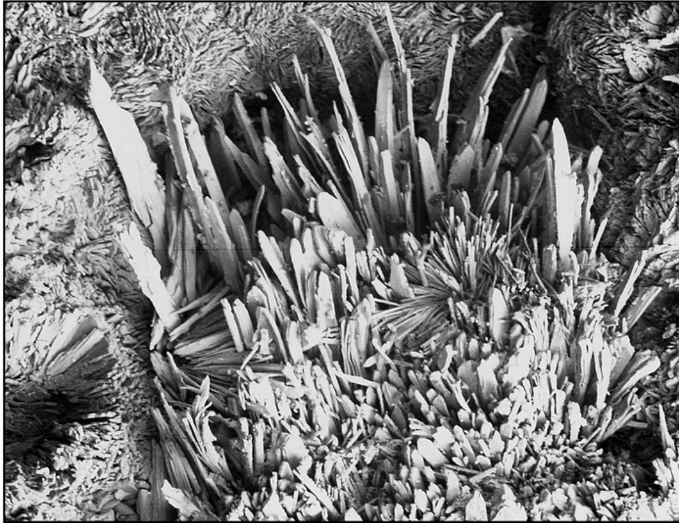
Figure 13. Mineral 21 with rosette of acicular macdonaldite crystals (field of view 2 mm). SEM photo by Gail Dunning.
