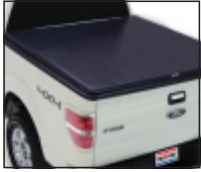
Press down rear cross member and push in on latch to open.
