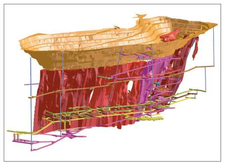
A 3D impression of Kemi mine showing the open pit, the underground development and the orebodies.
