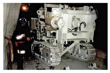
Diesel powered crawlers are used for transporting Robbins 34RH and Robbins 53RH.
