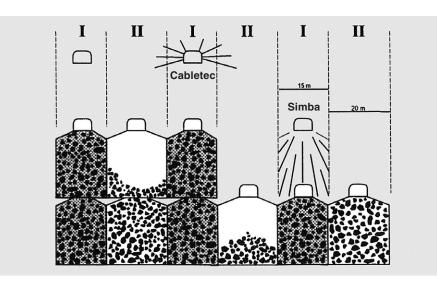
Cabletec drilling and installing cablebolts upwards, and Simba drilling blast holes downwards at Kemi mine.
