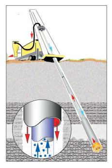
Principles for RC drilling showing flow of compressed air and chips. The sampling collection box is integrated into the cyclone.
