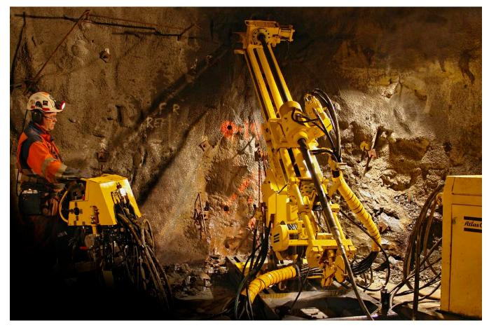
Atlas Copco underground core drilling rig Diamec U4.
