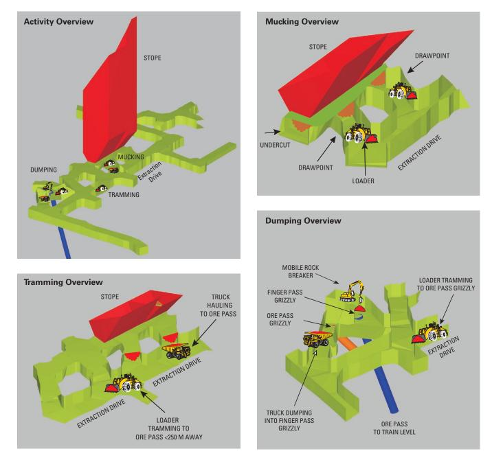
Activity overview showing mucking, tramming and dumping of ore from a typical stope.
