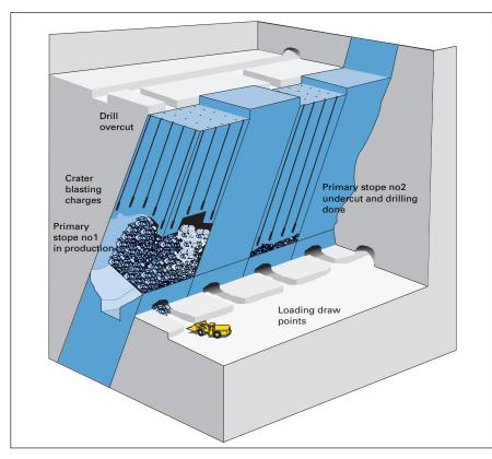
intervals. Nowadays, the loading level can be integrated with the undercut, and mucking out performed by a remote control LHD working in the open stope. This will reduce the amount of drift development in waste rock.
