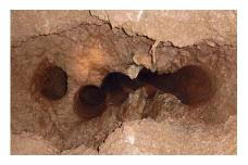
*Sufficient expansion space is created for production blast holes to follow.*
