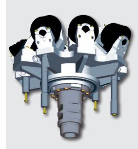
The 3.6 x 3.6 m operating limits at the mine work sites demanded an extremely low reamer design with a quickly detachable stinger. This reamer is bolted onto the machine when not in use. When piloting, the stinger is removed from the reamer, to allow the drill string to be fed through. In reaming mode, the stinger is refitted using the pipe loader, and the locking bolts are tightened manually.
