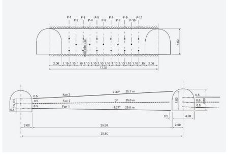
Undercut drilling to start the caving process.
