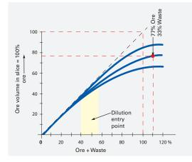
Typical ore/waste ratio during a mucking cycle. only. The hangingwall has to fracture and collapse, following the cave, and subsidence of the ground surface above the orebody has to be tolerated.
