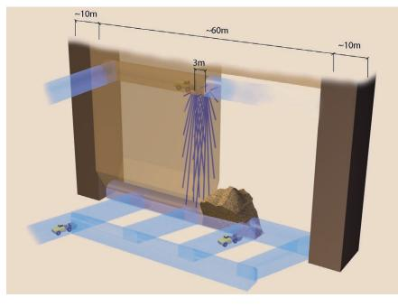
Schematic of sublevel stoping in a narrow vein using the Simba M6 C to drill down holes.
