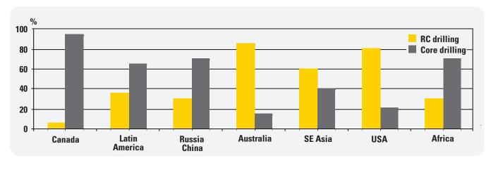
Ratios between core and RC drilling. The figures reflect total exploration expenditures from national statistics for surface and underground.
