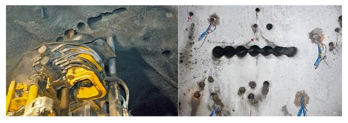
Slot drilling at Ferbasa: The Simba M6 C in action and, (right), the perfectly finished row of holes.
