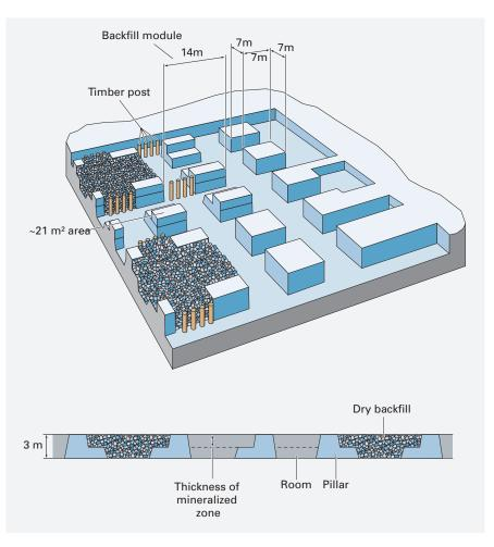
tricky, because the pillars in the first stage show a dangerous tendency for accumulation of energy. After 1983, the engineers in Rudna mine decided to adapt the dimension of the pillars to local geomechanical conditions. Also, alternating directions of driving stopes were introduced.
