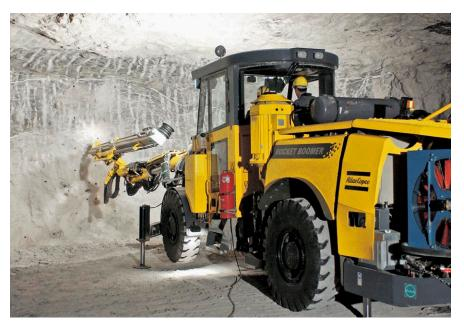
from 42mm bits, achieving a 2 m/min improvement in penetration rate, with accompanying gains in ANFO blast yield.
