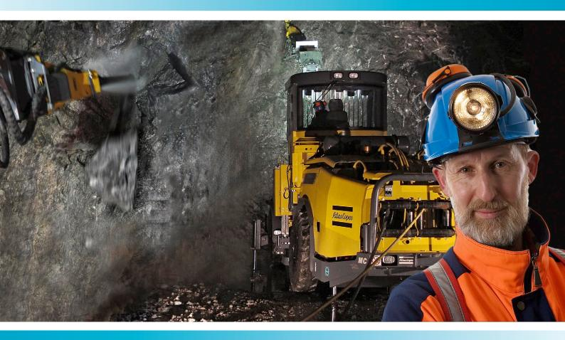
Add a solid body hydraulic breaker to a proven folding boom on the world's most tested underground carrier, and you have the Scaletec MC - a scaling rig for tunnelling and mining applications. Scaletec MC will give you higher productivity, less accidents, and take you a giant step along the route towards full mechanization.
