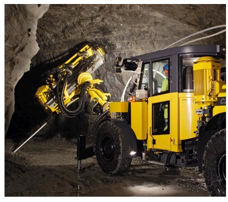
Mechanized cablebolting with Cabletec LC.
