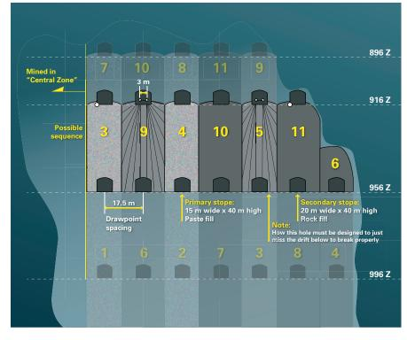
Sublevel stoping layout and mining sequence for Lappberget orebody.
