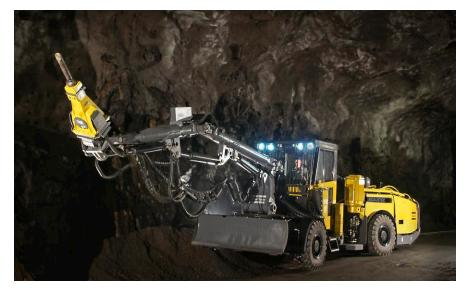
Mechanized scaling with hydraulic hammer
