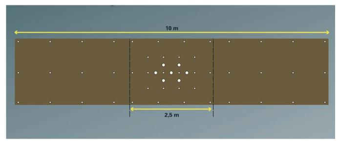
Drill pattern for cut off slot.
