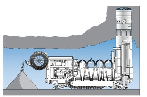
Typical operating installation of the BorPak machine.
