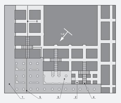
1. Back fill 2. Upper layer, extraction 3. Lower layer extraction 4. Ramp to lower layer 5. Water collector 6. Back fill piping
