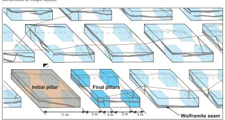
East-west oriented tunnels are called Drives, and those trending north-south are called Panels. Drives and Panels are driven 5 m-wide and, where they intersect, 1.8 m-diameter raises are bored between haulage levels to act as orepasses for all of the stopes. Chutes are installed in the bottoms of the orepasses to facilitate the loading of trains.
