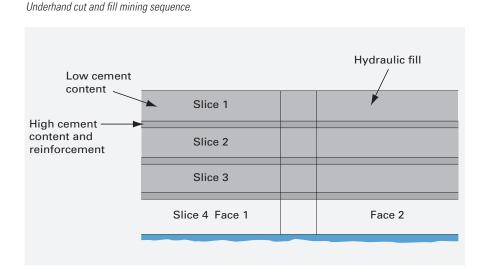
The first hydraulic fills were composed of concentrator tailings that would otherwise have been deposited on the surface. The mill tailings were cycloned to remove slimes so that the contained water would decant.
