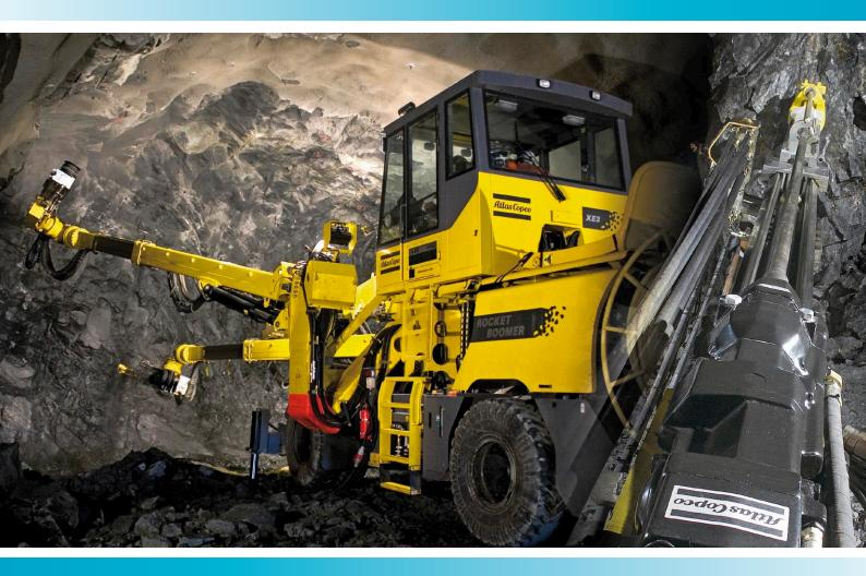
The Rocket Boomer E-series. A new face drilling rig that features the super-fast, prize-winning COP 3038 rock drill. It also introduces the BUT 45, a superb new boom that reduces hole deviation, provides extra large coverage area and slashes positioning time between holes by 50%. The result?
