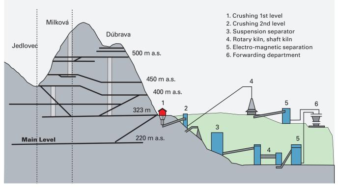
Idealised section of the mining operations and process plant at SMZ (Industrial Minerals).
