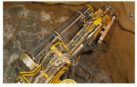
Boltec LC installing Swellex Mn12 rockbolts.
