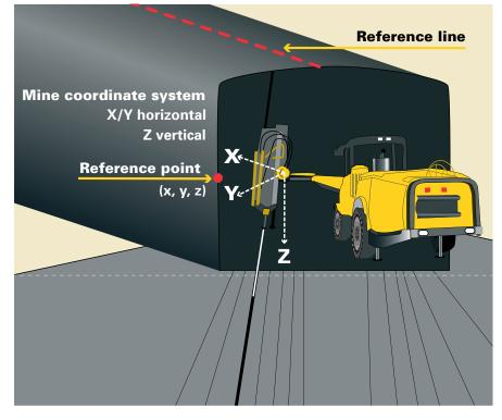
Navigation system for downwards longhole production drilling.
