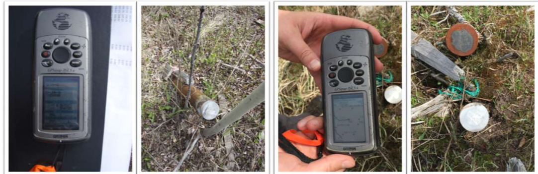
Figure 12.1 – Examples of on-site collar location verification (FAB-11-12 and FAB-11-26)
