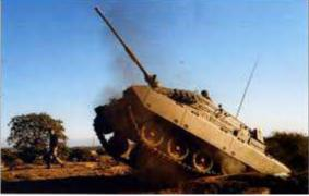
**FV-101 Scorpion**(Tier VIII Light Tank) A vehicle produced in 1972-which means that I've got my doubts that it will fit WoT timeframe-designed as an amphibious tank, capable of 80 km/h while carrying a selection of 30 mm, 76 mm or 90 mm guns, and lightened by the use of aluminum armor, it would be a perfect tank power-wise for the tier VIII gap.
