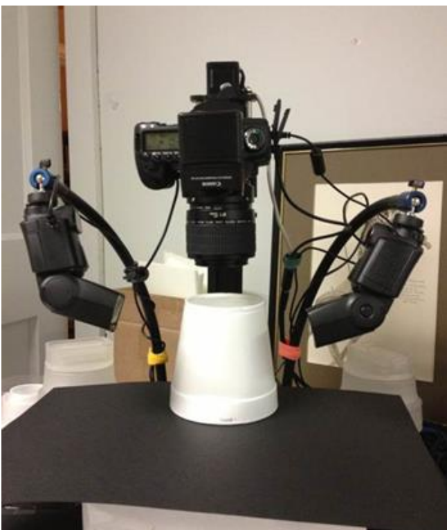
Figure 1. Styrofoam bowl acting as light diffuser. Visionary Digital Passport II setup. Photo by Chris Grinter
