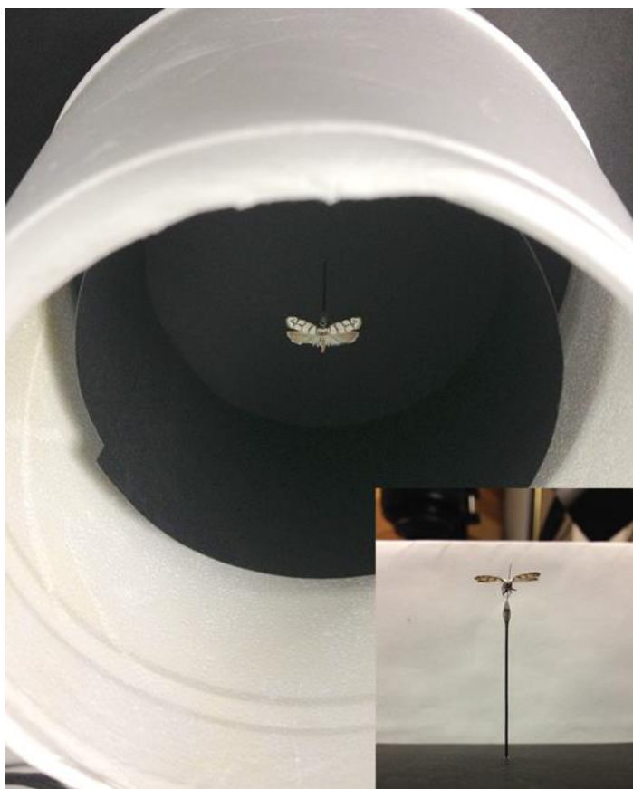
Figure 4. Top-down into my diffuser showing the black ring that helps to keep the flash from backlighting the specimen. Photo by Chris Grinter
