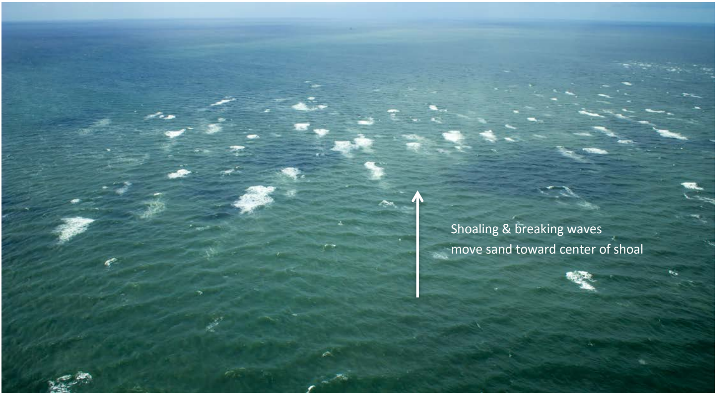
Figure 23. Breaking and shoaling waves across subtidal sand shoal. View is toward the west from the Gulf side.
