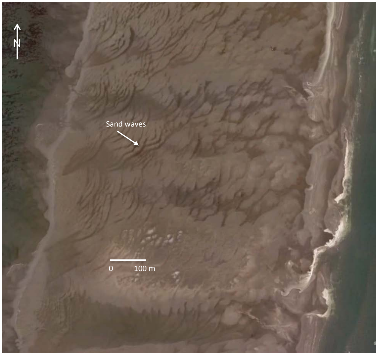
Figure 34. Vertical aerial taken on 29 October 2012. The photo demonstrates the impact of Hurricane Isaac that overwashed the barrier forming a broad washover fan that was subsequently reworked by waves and current from the northwest and formed 10-m wave-length sand waves.
