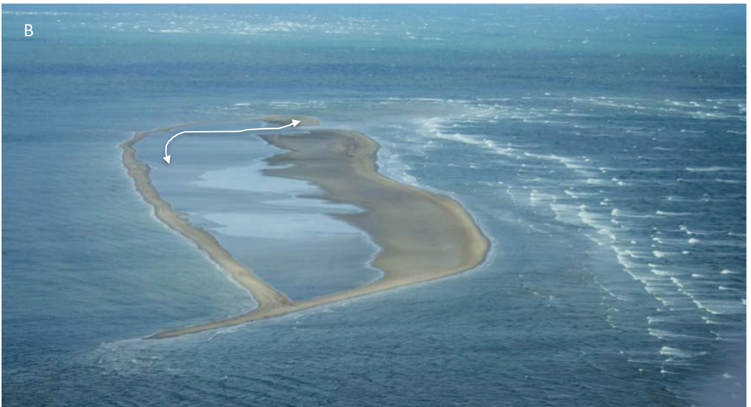
Figure 27. Newly developed barrier islands (A & B). Note the similarity of the two barriers with a more robust supratidal barrier on the Gulfside and a single thin bar formation on the bayside. The rise and fall of the tides produce tidal exchange (double arrow) keeping an inlet open at the north end of the incipient barrier.
