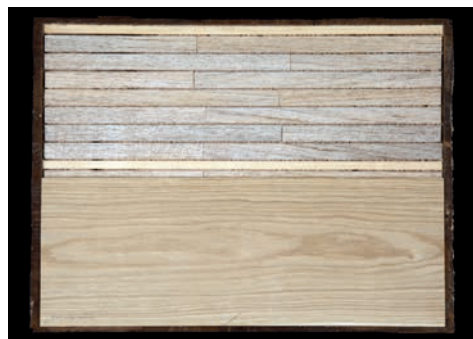
Fig. 17. The sandwich-like panel under construction. One half is already covered with thin oak board
