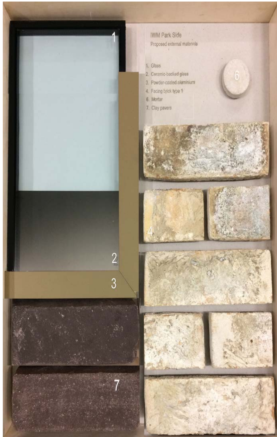
Figure 15: Physical samples of the proposed facing materials. Since the deferral of 18/AP/1577 at the 9 October 2018 Main Committee meeting, one of the materials (no.5, a brown facing brick) has been omitted from the design of the building; hence the absence of material no.5 from the above pallet.
