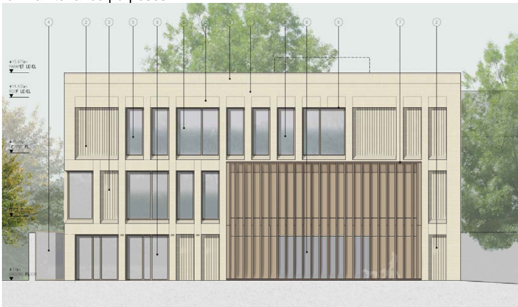
Figure 4: The southwest elevation of the proposed building, featuring a mixture of glazed (but fitted with graduated obscuring treatment) and brick-faced panels.
