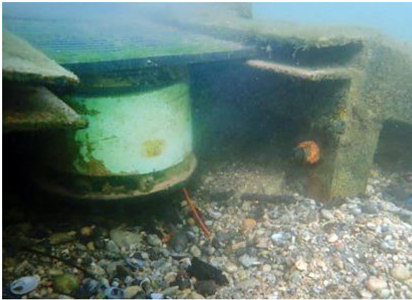
Figure 2. Custom bunker used in the study. Bunkers use the same principles as silos but are made to house larger adult mussels.
