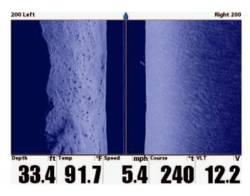
Figure 2. Side-scan sonar screen view of Alabama River substrate. The left side of the image shows boulder habitat along the channel slope potentially suitable for *Tulotoma*. The dark vertical column in the center of the image represents the water column. The right side of the image shows unstable sand substrate where *Tulotoma* are unlikely to be present.
