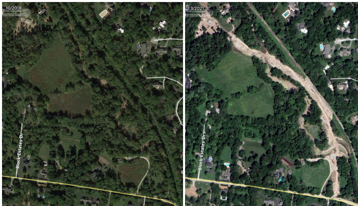
Figure 1. Before and after the 0.8 km (0.5 mile) MSD pipeline construction path on the property of the LREC. Left: October 2018, right: March 2021 (Google Earth 2019, 2021).
