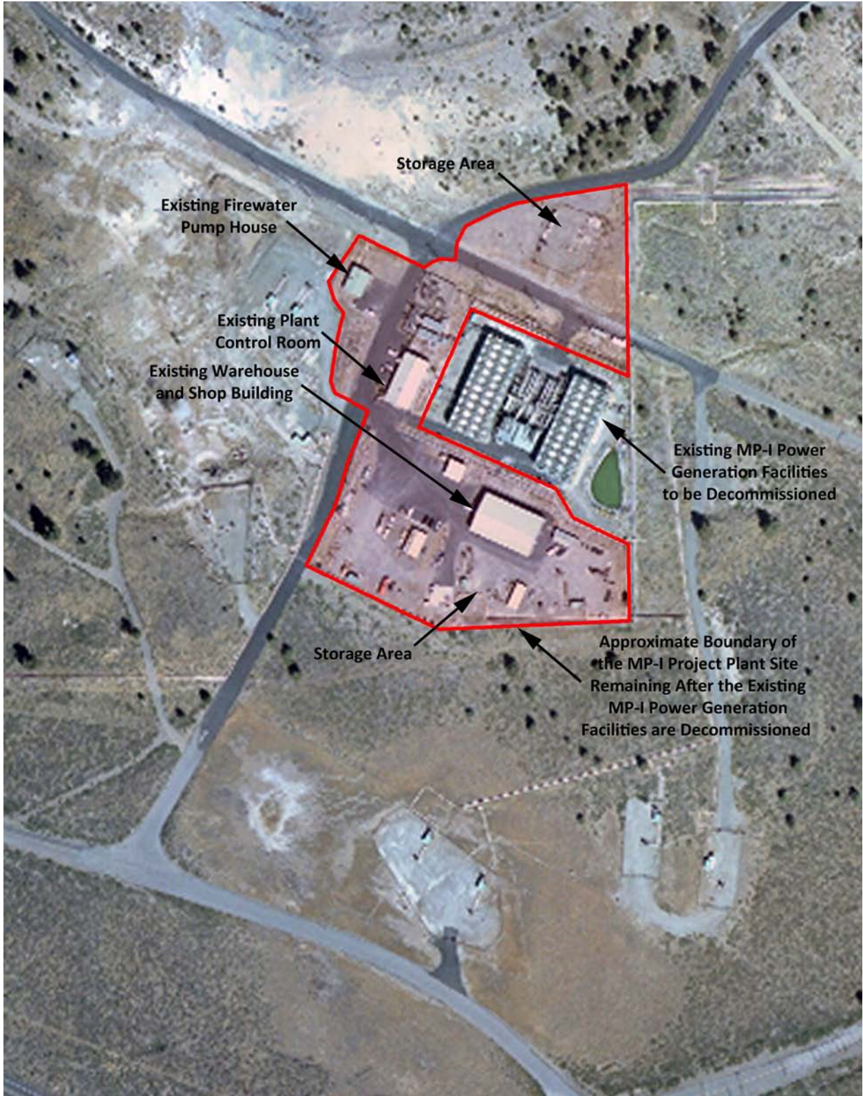
Figure 14: MP-I Project Plant Facilities and Areas that Would Not be Decommissioned
