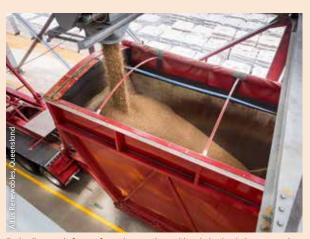
Fuel pellets made from softwood processing residues being loaded onto a truck for transport to the port of Bundaberg, Queensland, from where they are exported to European and Asian markets.
