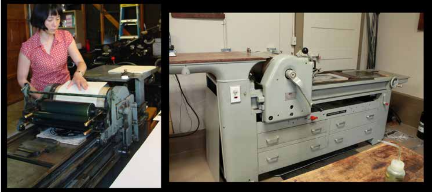
The Vandercook printing press has an inking mechanism with rubber rollers attached to the large impression cylinder that rolls over the blocks or type. It is hand-cranked and slow, but allows for leisurely pace of work.
