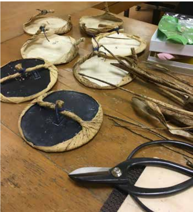
The baren, a burnishing tool, is the traditional means of printing block prints in Japan. Mr. Goto, the only known person known to make this tool in a strictly, time-honored way, teaches regular classes and workshops to disseminate his knowledge and techniques of making and maintaining this traditional tool.
