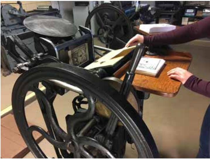
Starting with the Chandler & Price clamshell press we acquired a collection of more than a dozen old letterpress printing presses over two decades. This beauty with its graceful curved flywheel is a Gordon clamshell from the early 1900s.
