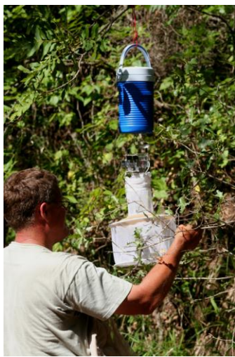
Figure 28. CDC light trap (Hausherr's Machine Works, Toms River, New Jersey) being checked in the morning.
