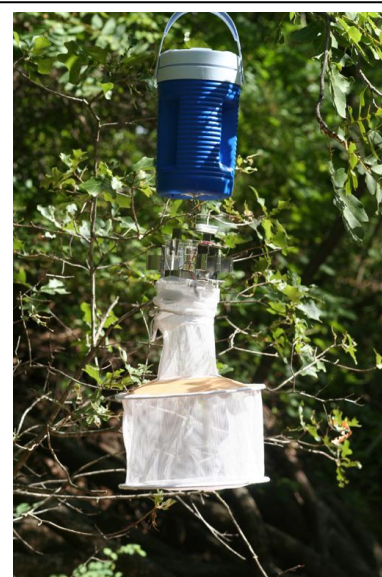
Figure 3. CDC light trap (Hausherr's Machine Works, Toms River, New Jersey). The blue drink cooler was filled with dry ice during the operation of the trap, and small holes at the bottom allowed the escaped of CO 2 to be circulated by the fan of the trap.
