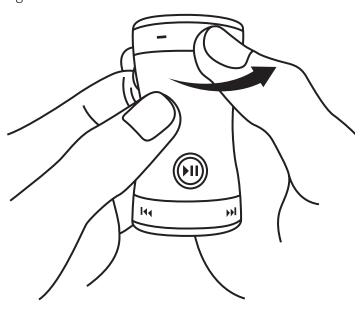
To turn down the volume, turn the **Top Twist** to the left. To turn the volume down fast, turn the **Top Twist** to the left and hold it.
