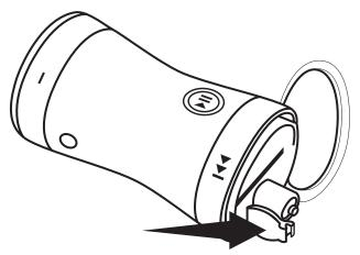
5) Close the battery cover Note: There should be a click sound when battery cover is closed properly.
