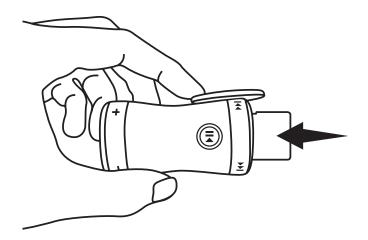
Note: The SD card's label must face down and the Sansa Shaker's Power/ Play/Pause button should face up while inserting the SD card.
