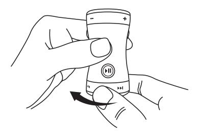
To rewind the current song, turn the **Bottom Twist** to the left and hold it.
