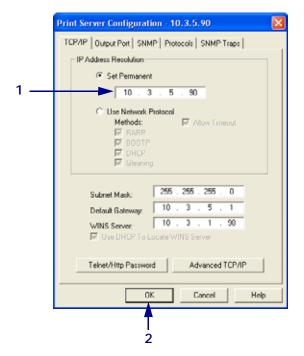
Set Permanent text-box. 2 **a.** In the Set Permanent text-box, type in the print server's IP address. **b.** When you are finished, click OK.
