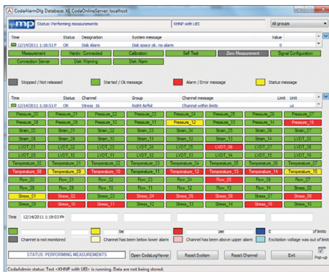
Alarm window: Full-featured alarm monitoring allowing the user to see the current status at a glance
