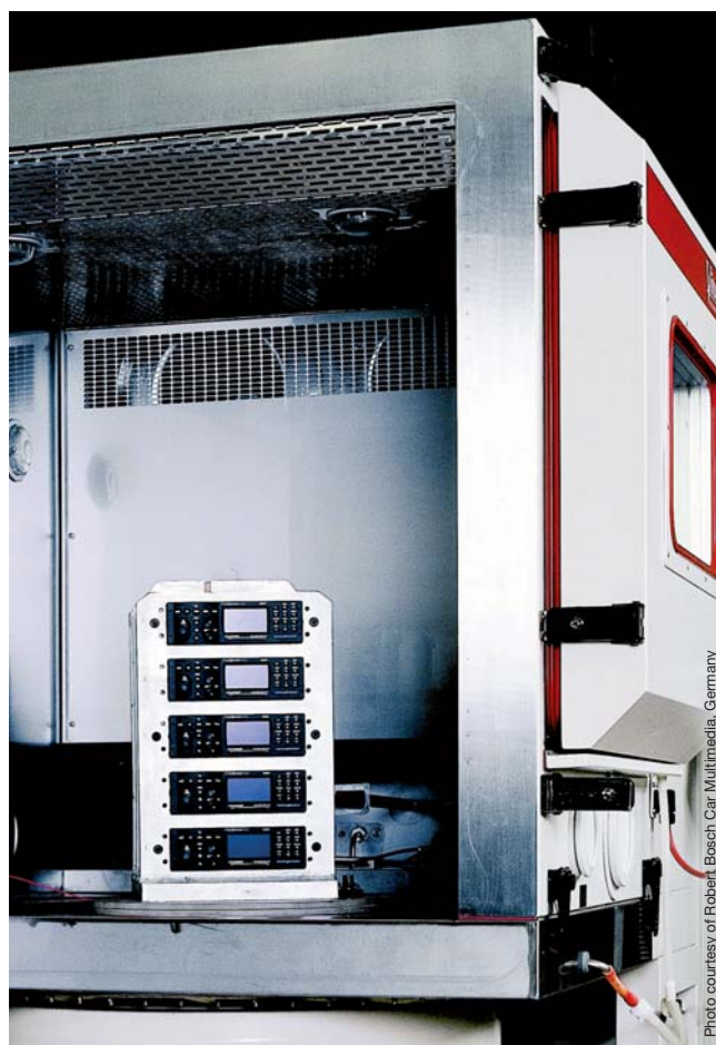
Combined climatic and vibration testing of car radios
