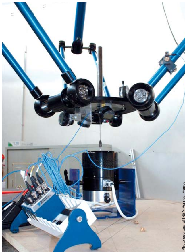
Modal analysis on a parallel robot
