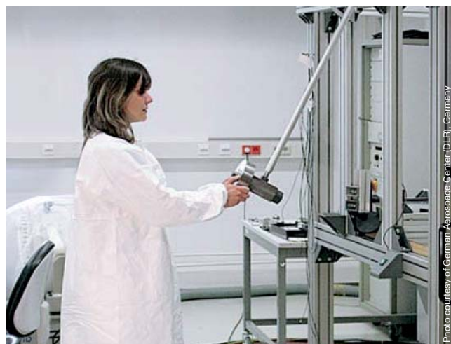
Shock Response Spectrum testing using an impact hammer
