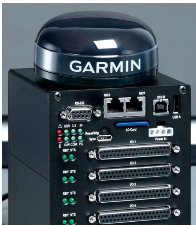
GPS receiver provides time and location information
