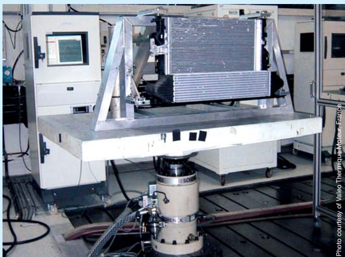
Testing engine cooling modules on a long-stroke shaker
