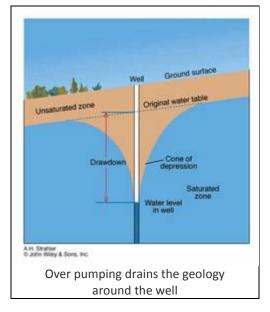
The rate at which water flows into your well is determined by the geology of the ground in which the well is constructed, the specifics regarding the construction of your well and the way that you operate it. How you operate a well can determine the quality and constituents of the water as well as the capacity and length of service the well will provide.
