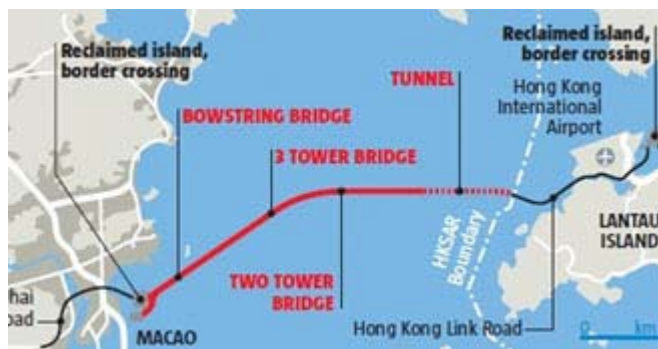
Hong Kong - Zhuhai - Macau Bridge Crossing
