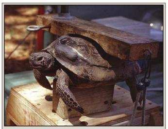
FIG. 3. Radio-instrumented Gopher Tortoise in the restraint device. Note both the eye bolt that allows vertical adjustment of the clamp to fit individual tortoises and the bungee cord that goes between eye screws on the clamp and base to further secure the tortoise.
