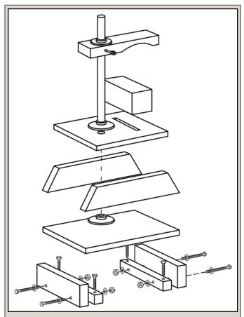
FIG. 1. Schematic illustration showing how parts of the tortoise restraint device come together.
