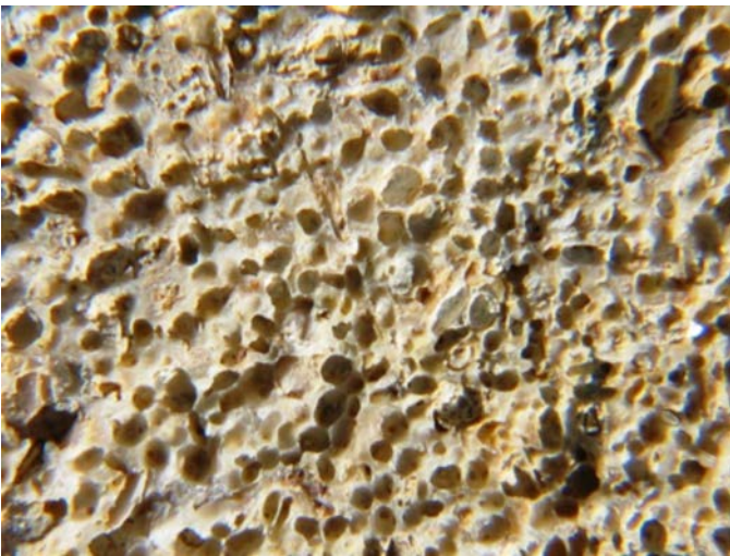
Close-ups of 4 different types of Jurassic limestone, all important stones for buildings and monuments. Each frame is c. 2 cm wide and shows what you would expect to see with a x10 magnifier and a clean surface. Fig. 1 (top left) Portland Stone with grain-prominent, small oololiths. Fig. 2 (bottom left) Bath Stone with spar-prominent texture. Fig. 3 (top right) Painswick Stone with most oololiths held tightly by the natural cement. Fig. 4 (bottom right) Dundry Stone with no oololiths, only shell fragments.
