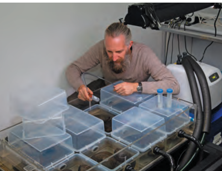
Figure 4 (below). Julian Finn tending the aquarium at Melbourne Museum. The containers with cobbles from Cumberland River are sitting in a clear tank. Stream water is pumped to this tank from a reservoir positioned below; inlet hoses can be seen at the lower right. The white box on the far right cools the water in the reservoir. The timer-activated light above the aquarium maintains the natural daylight cycle. A pooter is being used to catch adults. Photographer: Rodney Start | Source: Museums Victoria.
