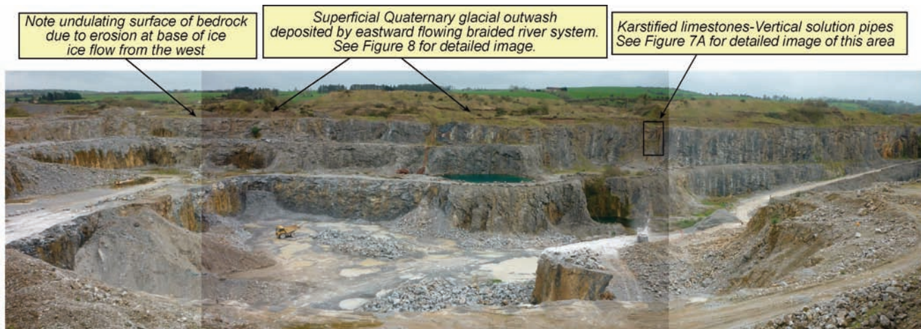
Figure 6. Locality 6 - View southwards across Castlemore South quarry showing Carboniferous Limestone bedrock unconformably overlain by Quaternary glacial outwash gravels and sands. The upper surface of the bedrock, the rockhead, is an undulating erosive surface which has been smoothed off by the passage of the easterly flowing Cork-Kerry ice sheet during the glacial maximum around 22,000 years ago. Brown staining in the bedrock is due to groundwater percolation through the limestone into the quarry. Note dumper truck and crane for scale.
