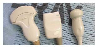
Figure 2.11. Three different probes. From left to right: Curvilinear abdominal probe, linear superficial probe, small-footprint cardiac probe.
