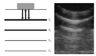
**Figure 2.8.** Reverberation echoes: (L) The sound beam travels between probe and strong reflector  $r_1$ . Artefact images  $r_2$ ,  $r_3$ , etc. are falsely generated. (R) How this appears in an ultrasound.
