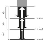
Figure 2.1. Depiction of the sound beam travelling from the transducer to the interface and back after reflection. The time until the sound returns depends on the distance to the reflecting interface — which means the travel time can be measured and converted into a distance.
