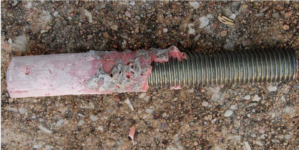
Figure 67. Post-Test Anchor Photograph, Test No. WEAB-14
