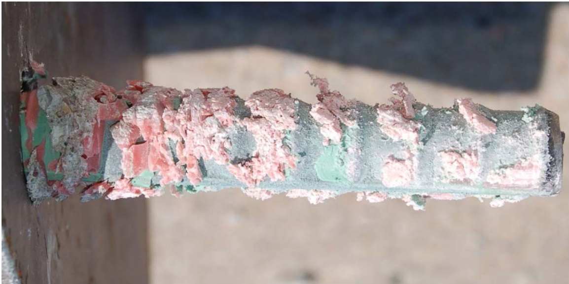
Figure 60. Post-Test Anchor Photograph, Test No. WEAB-12
