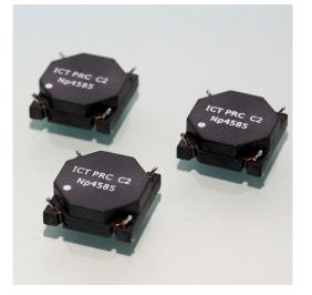
The ICT communications transformer series specially had been designed to meet customers requirement on high electrical performance with an extra low profile to be used in application with less space availability. These transformers are developed for the use with Echelon<sup>®</sup> TP/FT smart transceiver for LONWORKS<sup>®</sup> platforms. At a height of only 6,5mm it can be used in nearly all application.
