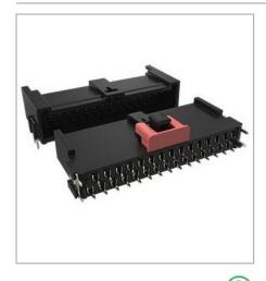
FlexLock®2.54mm FPC-to-board connectors are designed to address the growing demands of the automotive market. These compact USCAR-T2V2 compatible connectors have a nominal current carrying capacity of 3A per contact to support higher power application as well.
