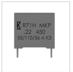
The R71H is constructed of metallised polypropylene film with radial leads of tinned wire. The radial leads are electrically welded to the metal layer on the ends of the capacitor winding. The capacitor is encapsulated in a self-extinguishing solvent resistant plastic case with thermosetting resin material meeting UL 94V-0 requirements. Automotive grade devices meet the demanding Automotive Electronics Council's AEC-Q200 qualification requirements.
