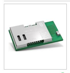
Panasonic has introduced the PAN1781, featuring the Nordic nRF52820 single-chip controller. The Bluetooth 5 features as the LE coded PHY for an elongated range or the high speed 2M PHY are supplemented by the support of Angle of Arrival (AoA) and Angle of Departure (AoD) direction finding using Bluetooth.
