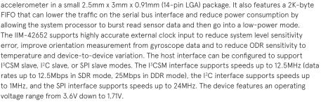
The IIM-42652 is a 6-axis SmartIndustrial™ Motion Tracking device that supports an extended operating temperature range. The IIM-42652 combines a 3-axis gyroscope, and a 3-axis
