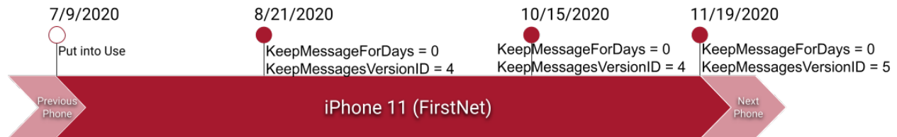
Figure 22 - A figure representing the presence and values of the “KeepMessageForDays” and “KeepMessagesVersionID” keys for the iPhone 11 (FirstNet)
