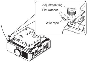
2) Pass the supplied flat washer (one) and wire rope through the adjustment leg (one) as illustrated on the left.
