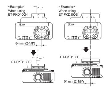
center of the attachment plate. However, when replaced with PT-DZ870, for example, the center position will shift to the left by 54 mm (2-1/8") as shown in the figure on the right.
