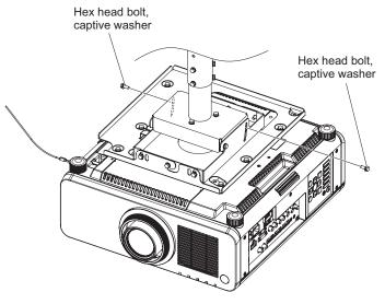
3) Use the two captive washer hex head bolts removed in the section "Removing the projector from the existing bracket" to secure the pole base (the attachment plate for a ceiling bracket for low ceilings) and the angle adjusting bracket as shown in the figure on the left.
