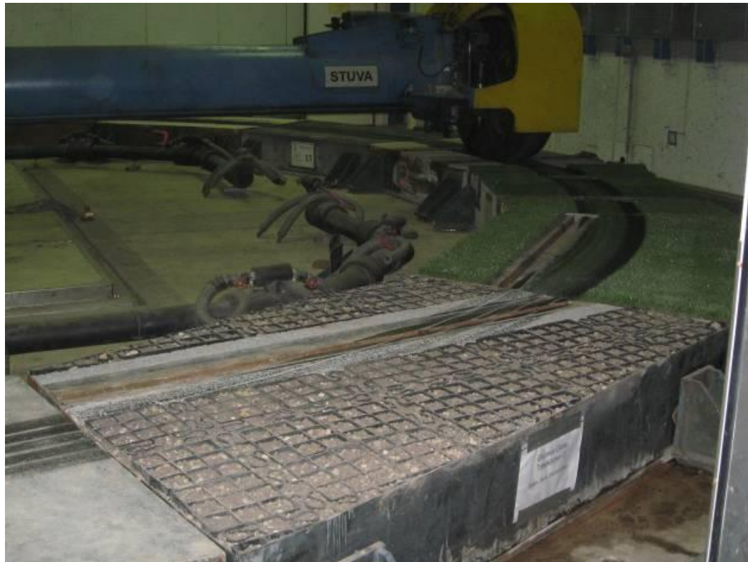
Drain concrete test body at STUVA fatigue laboratory, after testing
