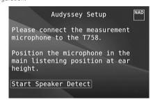
The sound at your main listening position is setup using the supplied Audyssey microphone. A special test tone is sent to each speaker and the data is memorized by the T 758. The duration of setup may take some time depending on the number of speakers. After the measurements, Audyssey calculates the ideal system response for your particular room and speaker setup.
