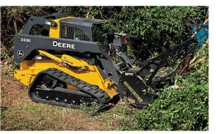
Photo 2. Skid steer with masticating/mulching attachment.
