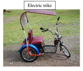
Because of our experience with designing electric cycle rickshaws we designed two rickshaws for handicapped persons. One was a Motor Assisted NARI Handicapped Rickshaw (MANHARA), and the other was a completely automated rickshaw called an electric trike. Both have been given to few handicapped persons. An excellent
