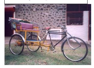
We then designed a lightweight and easy-to-drive rickshaw and tested it Phaltan on roads. However, converting this improved rickshaw into an electric-powered one proved to be quite difficult, since in those days 1990s) (mid small, high-torque permanent magnet D.C. (PMDC) and controllers were not motors
