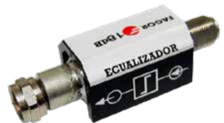
Fagor 15 db Equaliser covering 47 - 862 MHz. 1 dB insertion loss at 862 MHz
