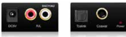
Blustream DAC (Digital to Analogue Audio Converter) converts either digital optical or coaxial to analogue stereo left/right audio output
