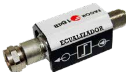
Fagor 9 db Equaliser covering 47 - 862 MHz. 1 dB insertion loss at 862 MHz
