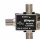
PIK2400 Power Injector, 60V 2A Max. (F31017)
