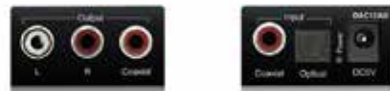
Blustream DAC (Digital to Analogue Audio Converter) converts either digital optical or coaxial to analogue stereo left/right audio output
