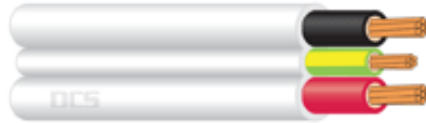
CMTE-2.52C+E - 2.5 mm Copper Core, (TWIN+Earth) Red and Black + Earth PVC V-90 insulation Cores - 100m roll
