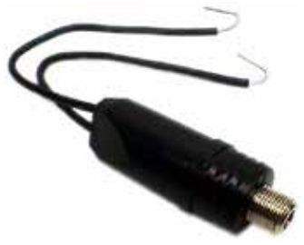
300 ohm to 75 ohm with Moulded Plastic Balun Housing and Solid Core Wire Inputs and F Connector Output
