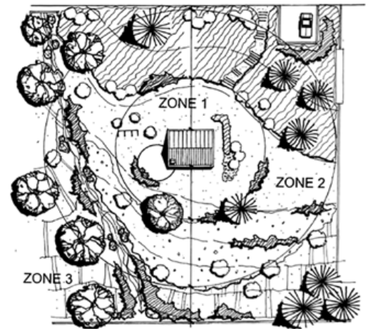
Firescaping with three zones around a house or structure to increase fire-resiliency: Zone 1 extends from the structure to 30 ft., Zone 2 is 30 to 70 ft., and Zone 3 is 70 to 120 ft. Illustration from Richard Kent's book Firescaping (Wilderness Press 2005).
