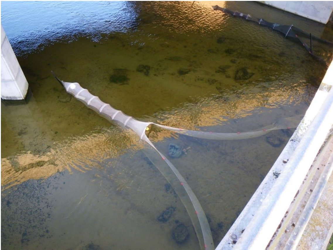
Larval (green) and standard (white) directional fyke nets (top) and close up of larval net showing finer stretch mesh on funnel (bottom left and right)
