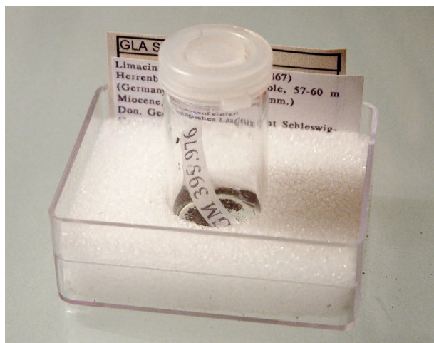
Fig. 10. Storage of pyritised pteropod samples in silicone oil, in upright glass vial, in polystyrene container, with labels separated, in standard RGM collection box.
