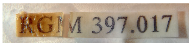
Fig. 11. Label attacked by pyrite disintegration, kept in vial with silicone oil.
