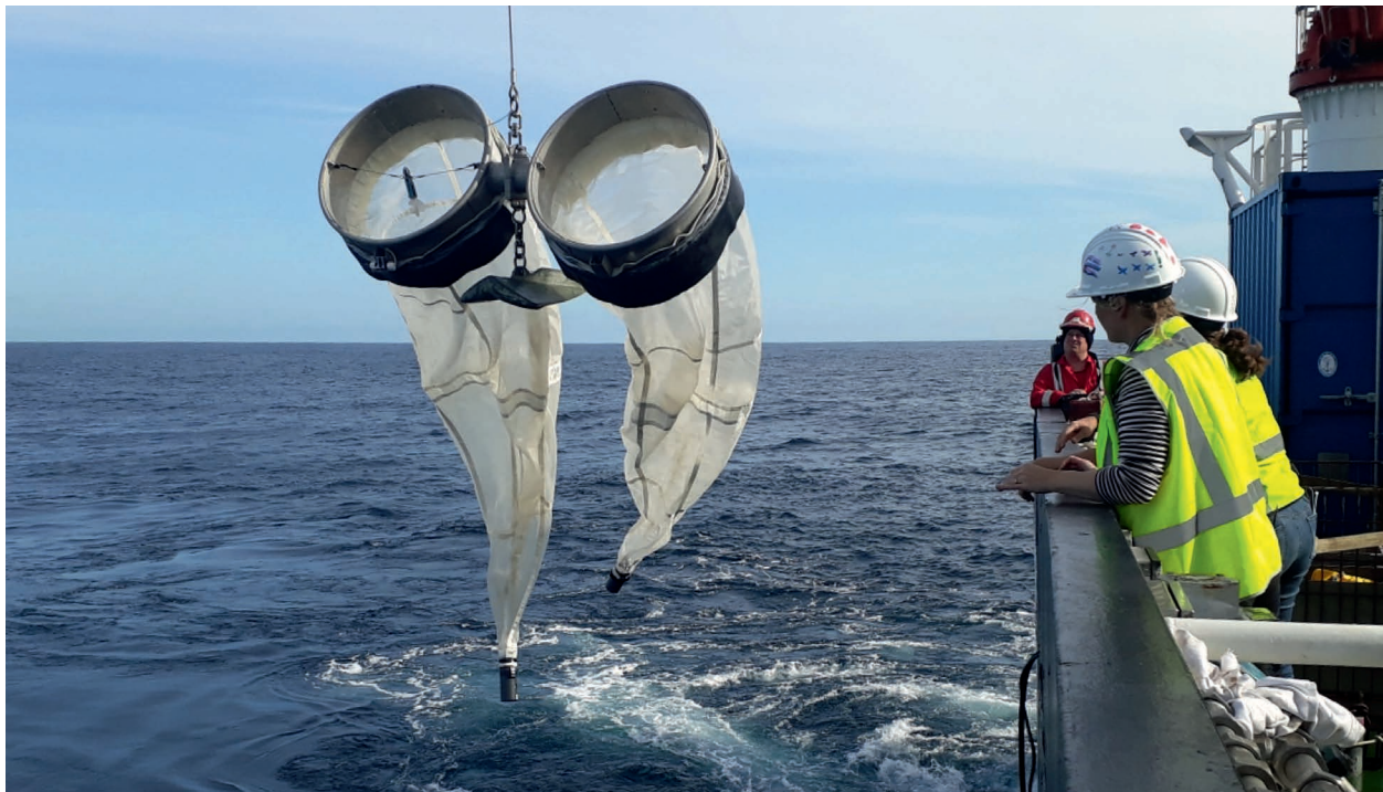
Fig. 7. Sampling of zooplankton with a Bongo net during Atlantic Meridional Transect 27 in 2017.
