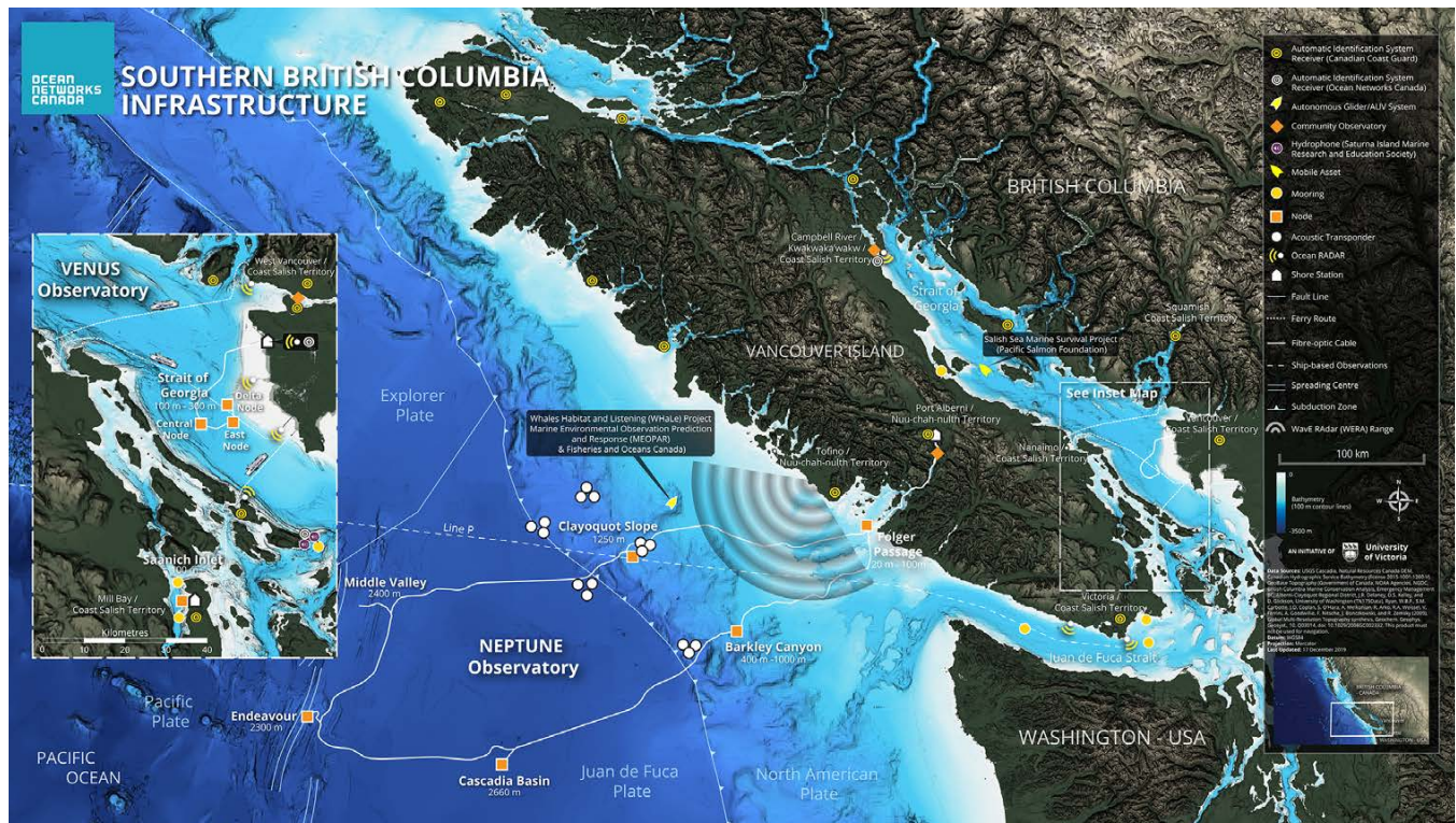
FIGURE 1. A map of Ocean Networks Canada’s (ONC’s) Southern British Columbia infrastructure. The white dots represent the locations of the acoustic transponders surveyed by a wave glider as part of the Northern Cascadia Subduction Zone Observatory.
