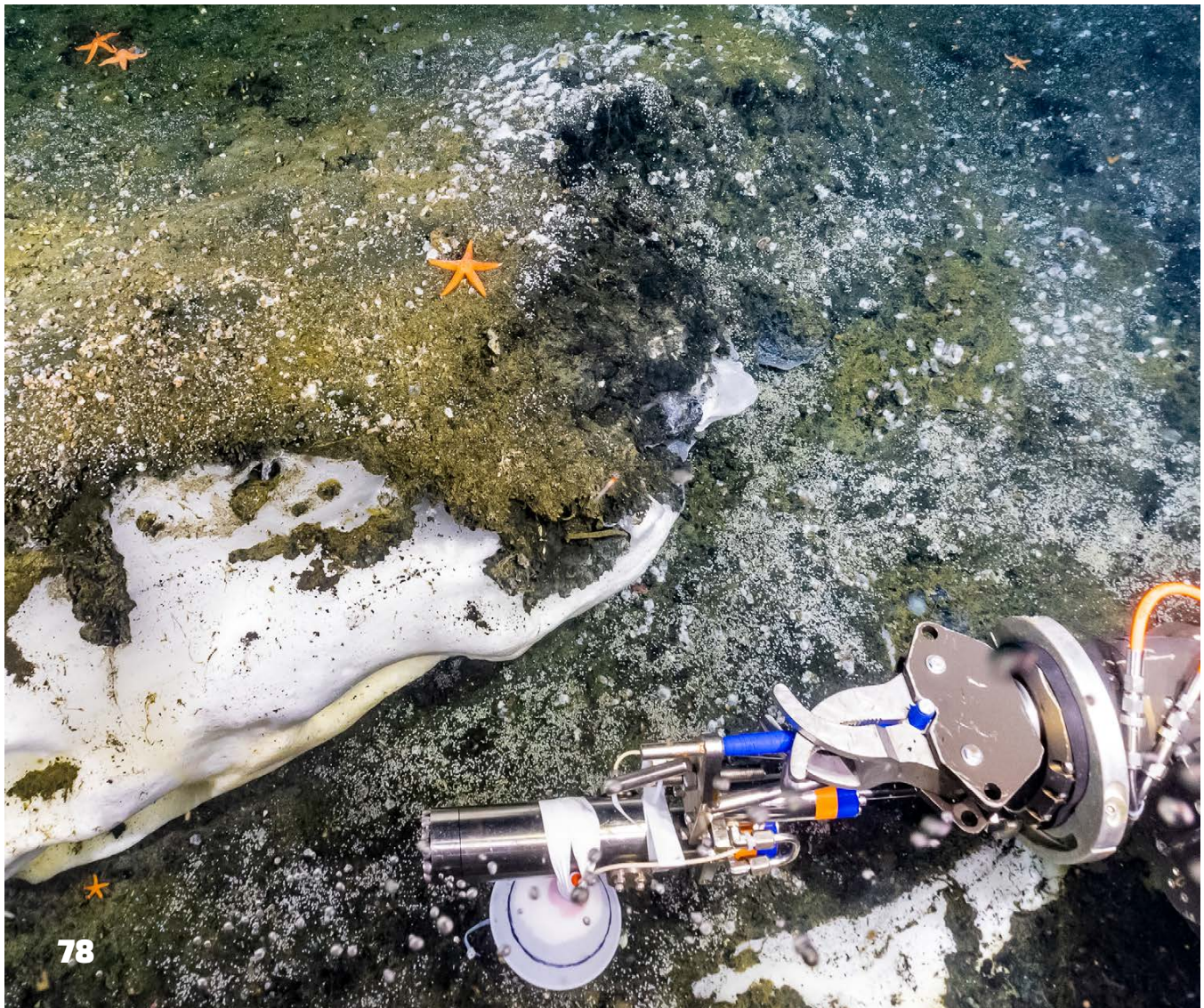
Methane seep bubbles are seen floating in the foreground as ROV Hercules pilots operate a gas-tight sampler along the Cascadia Margin during E/V Nautilus expedition NA128. Image credit: OET
