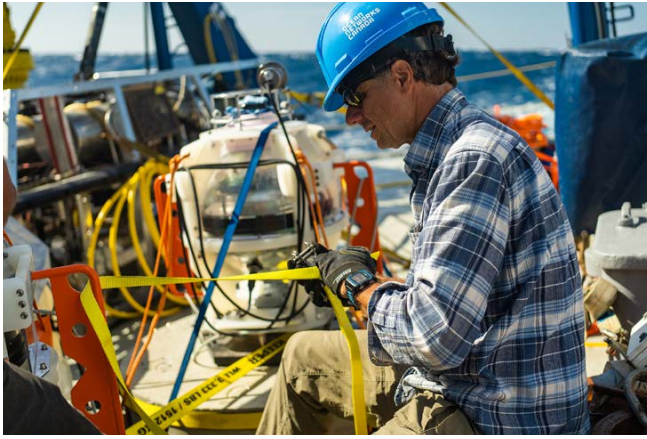
FIGURE 2. ONC's Director of Observatory Physical Operations Ian Kulin prepares to deploy a Sonardyne FETCH transponder to measure tectonic plate movement to centimeter accuracy as part of the Northern Cascadia Subduction Zone Observatory Project.
