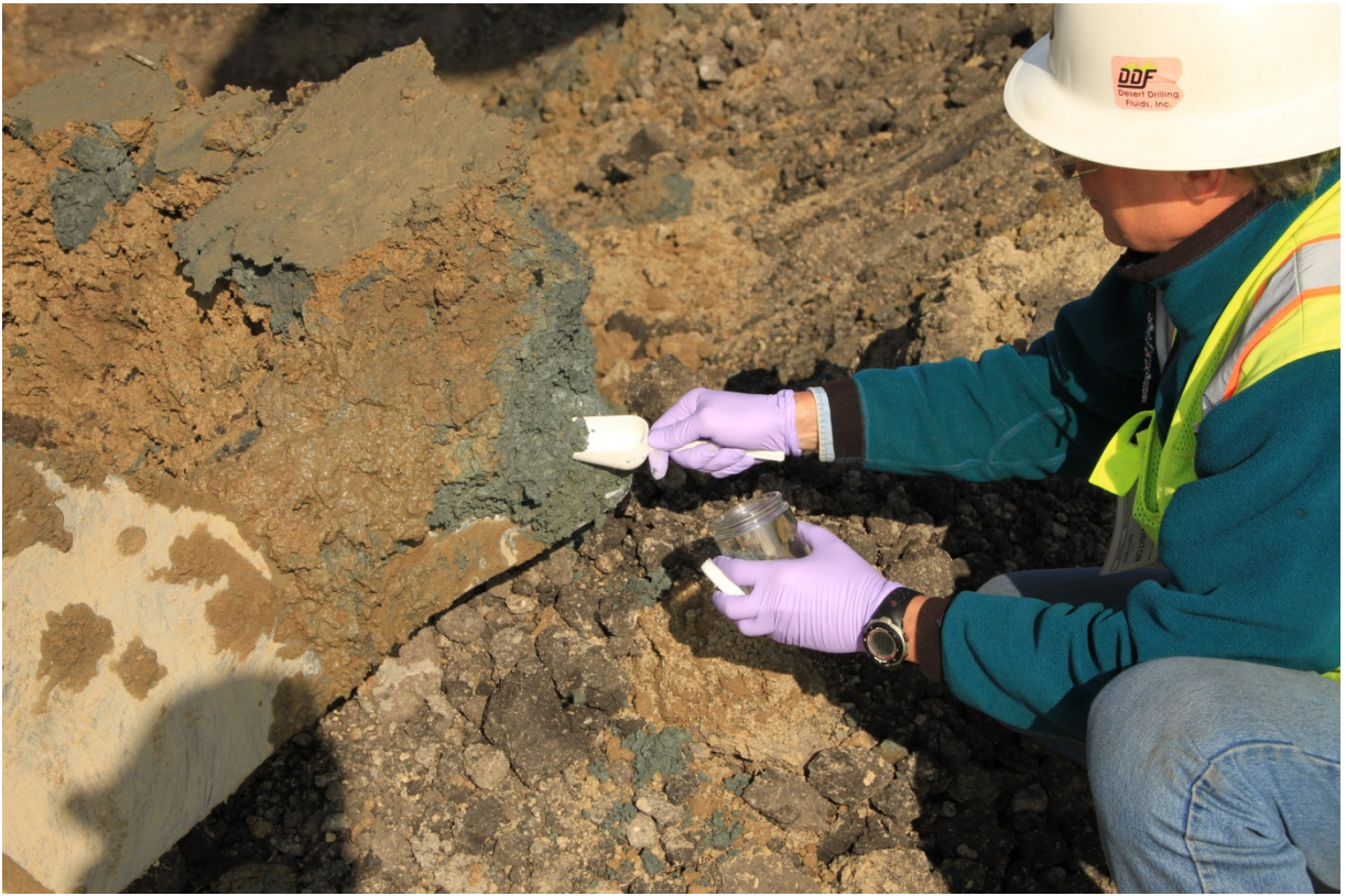
Photograph D-5. Collecting sidewall sample
