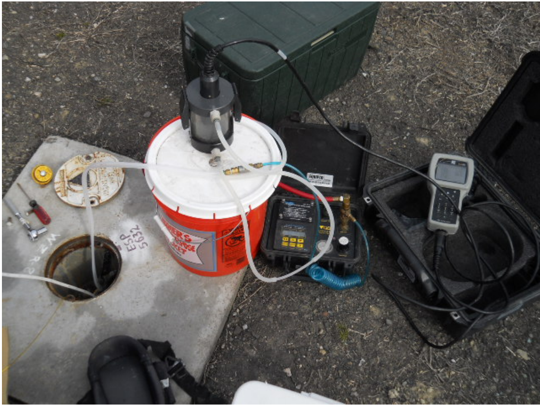
Photograph D-21. Well purging and parameter monitoring before sampling
