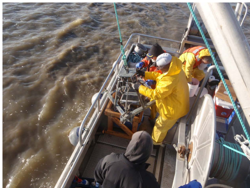
Figure 3. Illustration of sediment collection using stainless steel, 0.1 m 2 Smith-Macintyre sediment grab sampler. (Note water turbidity.)
