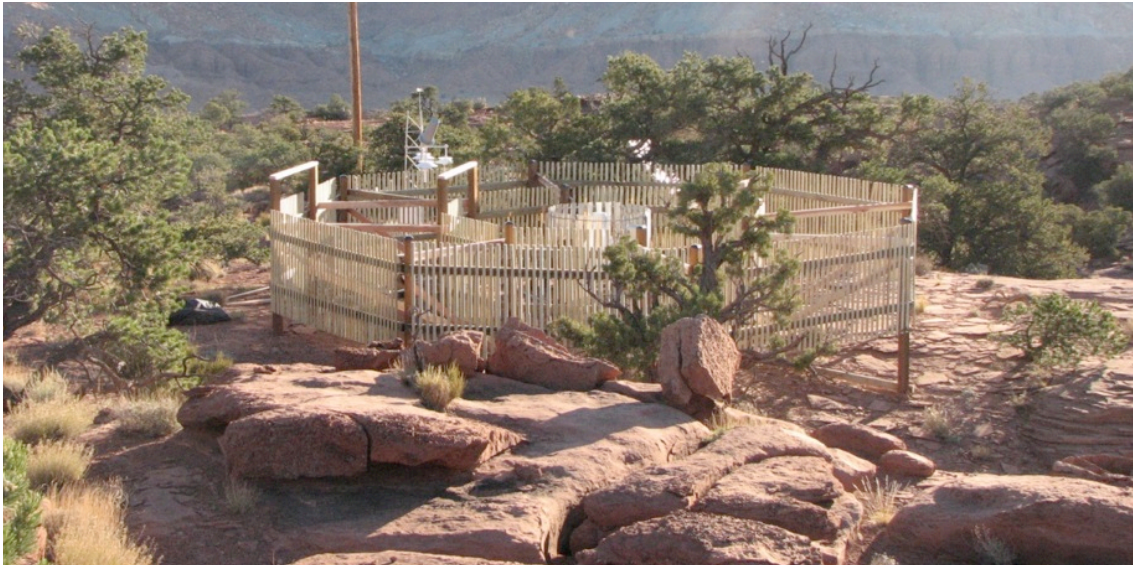
Figure 2: Photograph of well-shielded Geonor rain gauge showing both wooded SDFIR and metal double alter shields at the USCRN station in Torrey, Utah.
